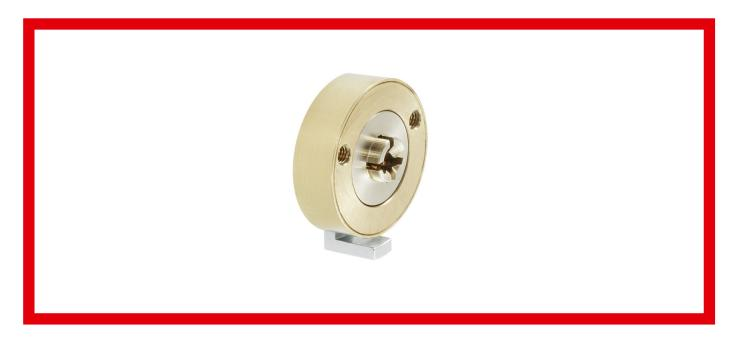
As variants of IKON pin cylinder systems, cross profiles provide security in the smallest of spaces. Rows of pins on three corresponding sides with minimal installation dimensions provide effective protection against manipulation. Cross profile locks are also available on request with a special paracentric profile. Suitable keys for concealed installation are available in different lengths from IKON.
