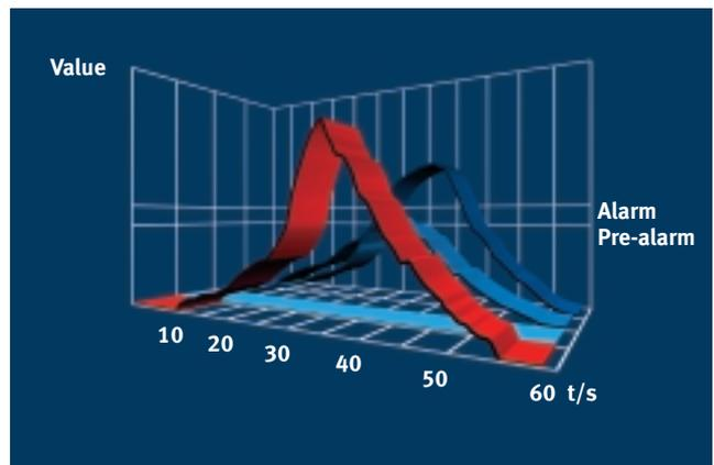
*With light smoke the O<sup>2</sup>T detector triggers an alarm sooner than normal scattered-light detectors*
