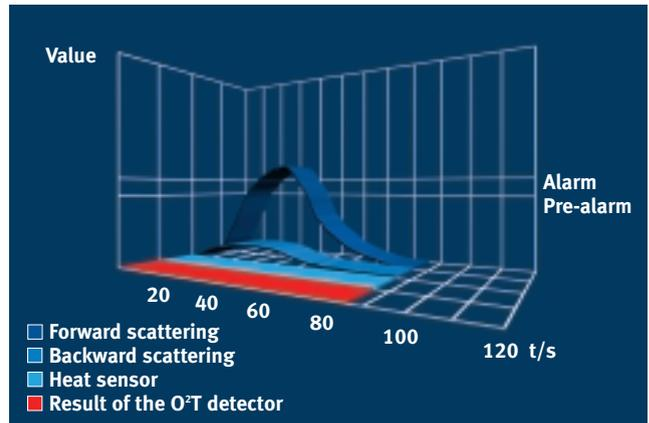
*Unlike normal scattered-light detectors the O<sup>2</sup>T gives no alarm with steam*
