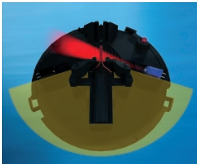
*The O<sup>2</sup>T detector operates with 2 light reflection angles. The detector optimises the measurement of forward and backward reflections identifying without compromise all types of smoke and greatly reduces false alarms.*
