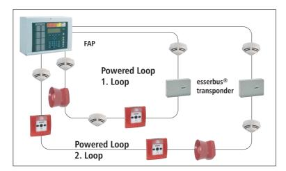
The sensors of intelligent multisensor detectors in the esserbus<sup>®</sup> can be switched on and off manually or by a timer. The esserbus<sup>®</sup> transmits not only detector alarm signals but also detector maintenance instruction and warning signals. In addition, the location of each detector on the bus can be accurately assigned with a convenient text display.
